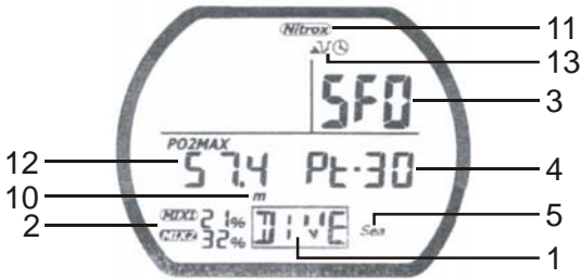
Dive option display and set fields for screen one
