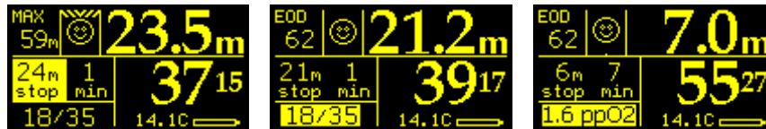
Deco ceiling violation warning, Mix swap reminder, 1.6 ppO 2 warning shown when exceeding that level,
