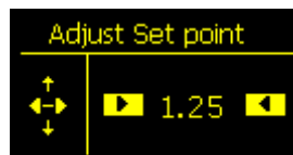
Underwater set point adjustment. Scroll up down to adjust, left right to accept.
