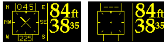
Left: X1 orientated to a heading of 045 degrees. Right: blank display when X1 is tilted too far from horizontal.
