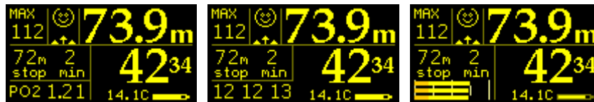
Three ways to display PO2 information: Hi cell, 3 cells or bars (1.2 shown).
