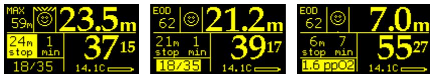
Deco ceiling violation warning, Mix swap reminder, 1.6 ppO 2 warning shown when exceeding that level,
